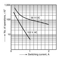
3. Contact reliability for AC loads Tested sample: DS2E-S-DC24V 10 pcs. Operating speed: 20 cpm. Detection level: 200 m $\Omega$
